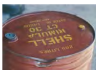
Figure D2: Reprocessing steel drums – chime and head damage
