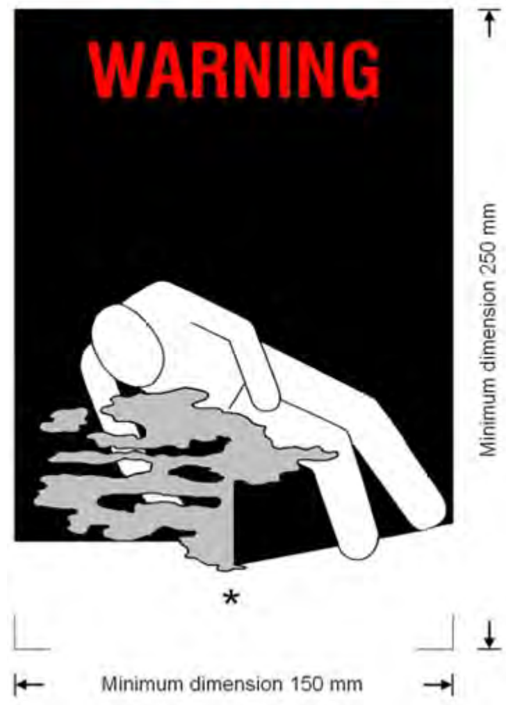
Figure 5.5.2: Asphyxiation warning mark for cargo transport units
