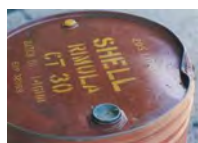
Figure D2: Reprocessing steel drums – chime and head damage
