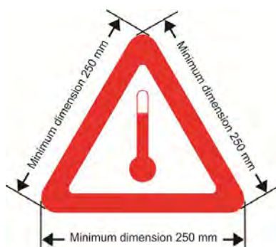
Figure 5.3.4: Mark for carriage at elevated temperature
