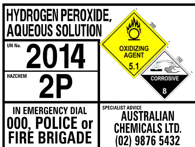
Figure 5.3.2(c): Examples of Completed Emergency Information Panels
